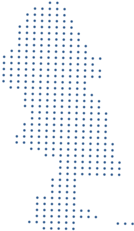
Figure 7. Example of spatial sample organization based on grid stations
